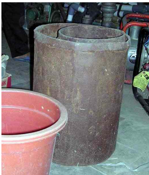
Gambar 7a. Ring infiltrometer ganda
